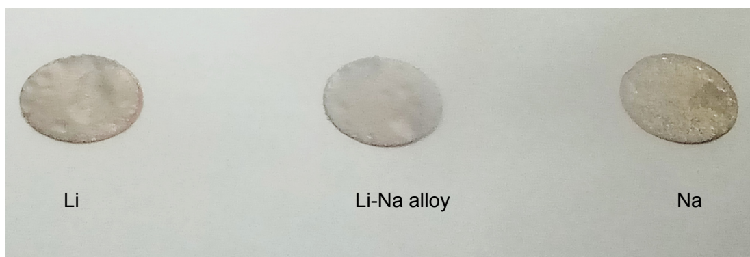
Supplementary Fig. 4. The photos of plated Li, Li-Na alloy, or Na metal on Cu foil. The plated capacity is 3 \text{ mAh cm}^{-2} at a current density of 0.5 \text{ mA cm}^{-2} .
