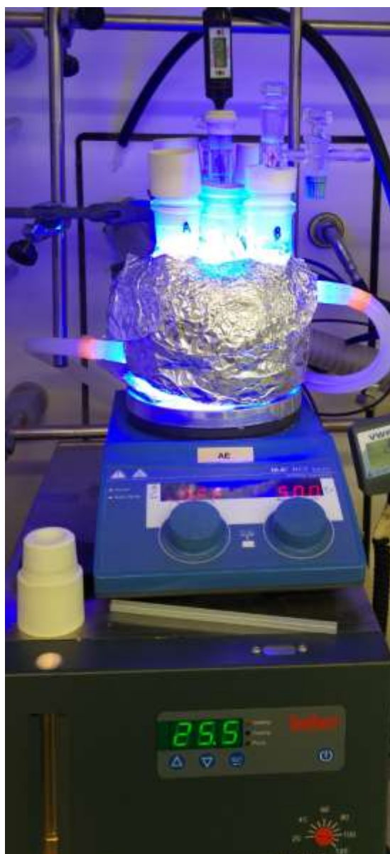
Supplementary Figure 4: Fully assembled photoreactor in operation.
