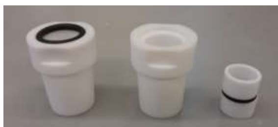
Supplementary Figure 3: Teflon adaptors used to accommodate Schlenk tubes in the photoreactor.
