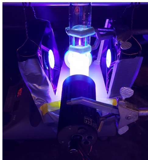
Figure S6. Gram-scale synthesis using 2 Kessil® LEDs at 100% power with 2 fans facing each other for cooling
