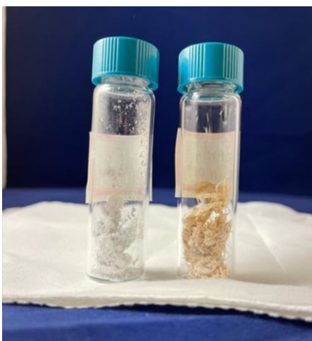
Figure S20. Photo of dPVC recovered from reactions performed using PVC 47k with 1 equiv. of DEHP (dPVC DEHP , left) and with no DEHP (dPVC alone , right).
