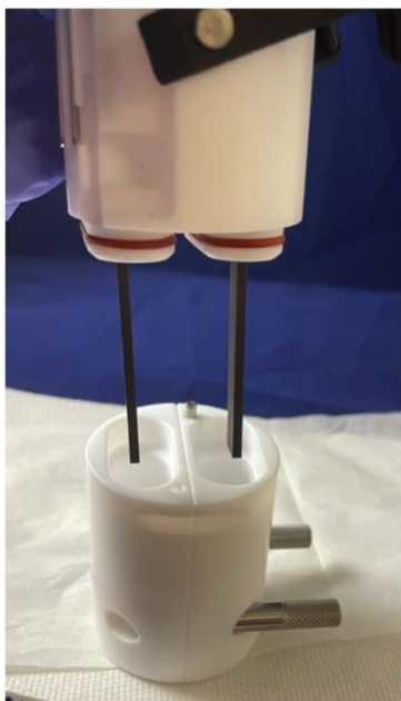
add reagents (not shown) and Pro-Divide cap with electrodes
