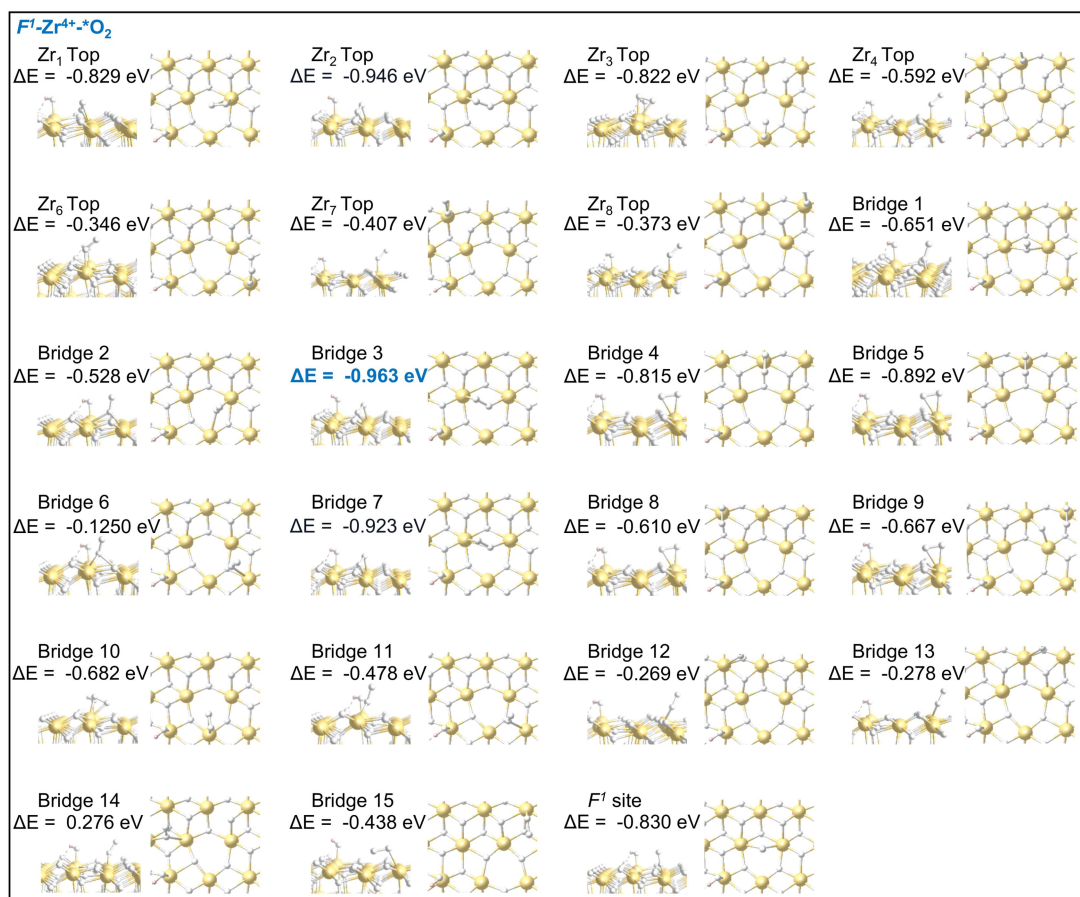
Supplementary Figure 54. Optimized geometric structures and corresponding calculated energies for ^*\text{O}_2 intermediates adsorbed at different sites on the F^I\text{-Zr}^{4+} .
