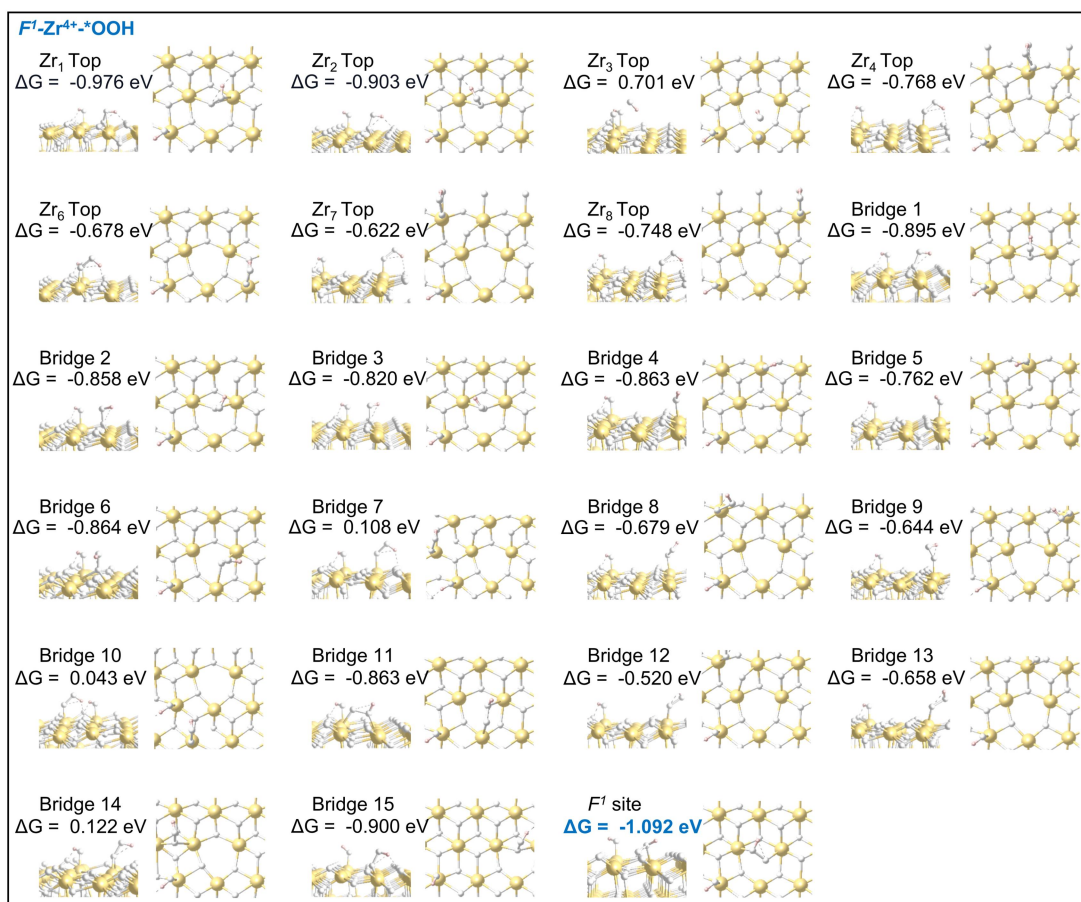
Supplementary Figure 55. Optimized geometric structures and corresponding calculated energies for *OOH intermediates adsorbed at different sites on the F^I\text{-Zr}^{4+} .
