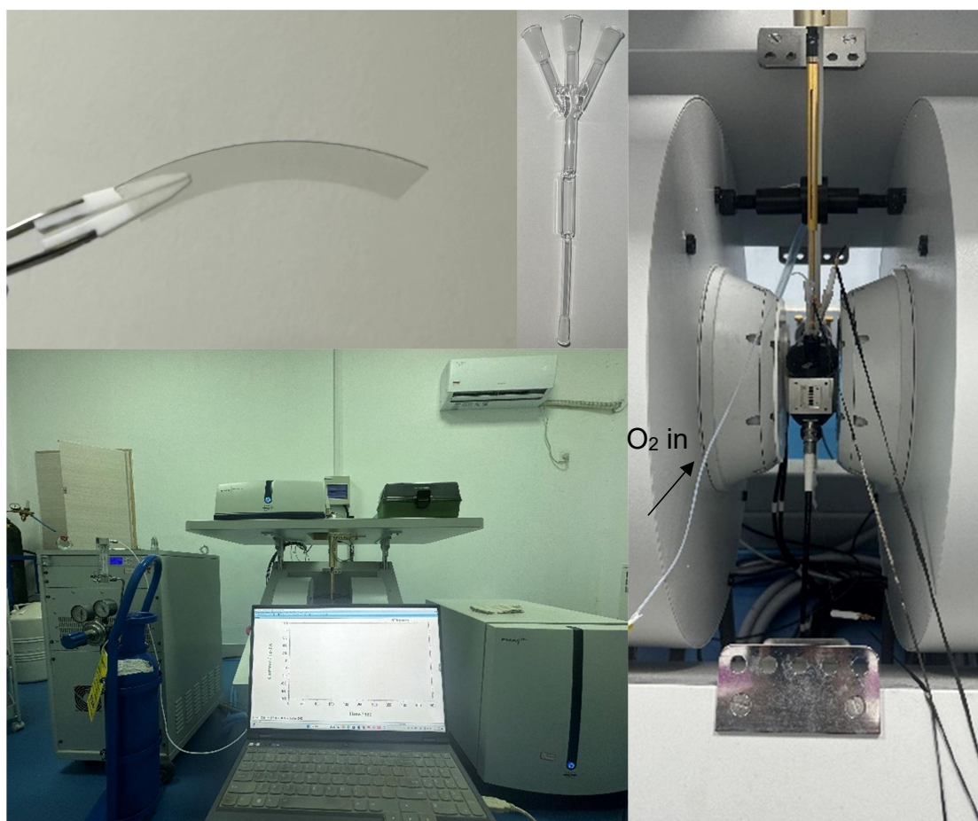
Supplementary Figure 34. Photograph of the in situ EPR setup for electrochemical ORR testing.
