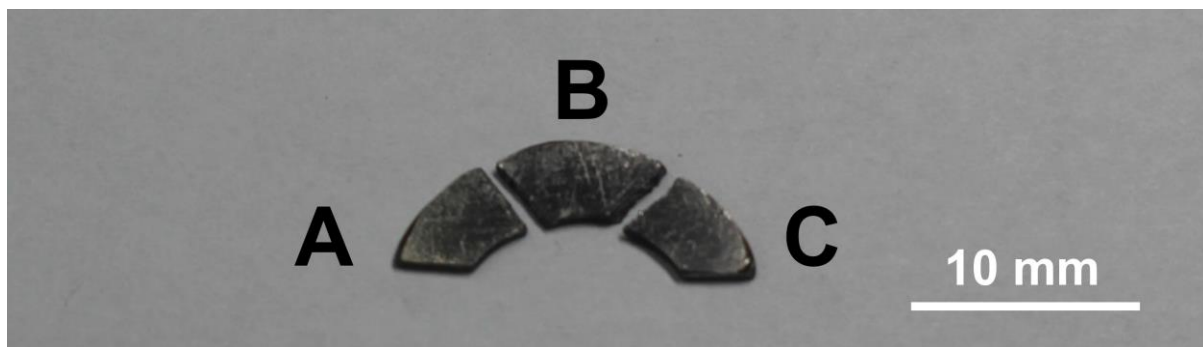
Supplementary Figure 7 | Three different pieces cut from the same half-ring for measuring TE properties.
