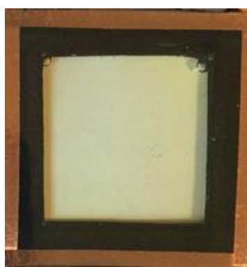
Supplementary Figure 11: Photograph of a 25 cm 2 dynamic window utilizing an unmodified ITO counter electrode. Following 10 complete cycles of -2.5V for 30 s and 0V for 60 s, the device turns yellow due to the formation of Br 3 - in the electrolyte.
