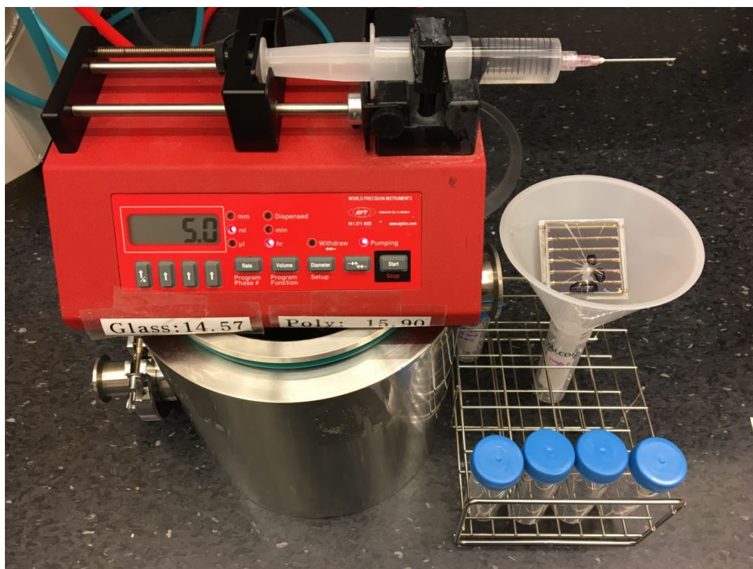
Supplementary Figure 10 | Photograph showing the water dripping test. Acid water ( \text{pH} = 4.2 ) was continuously dripped at the damaged part of the perovskite solar module at a speed of 5.0 \text{ mL/h} for 1.5 \text{ h} to simulate a heavy acid rain after the perovskite solar module is damaged by natural causes (e.g., hail impact).
