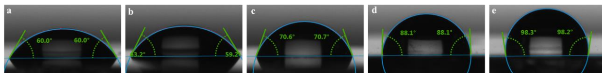
Supplementary Figure 1. Water contact angles for perovskite films with different alkyl chain length AALs. a-e, Water contact angles of the pristine CsFAMA film ( a ) and the CsFAMA film with BA ( b ), PEA ( c ), OA ( d ), and OAm ( e ).
