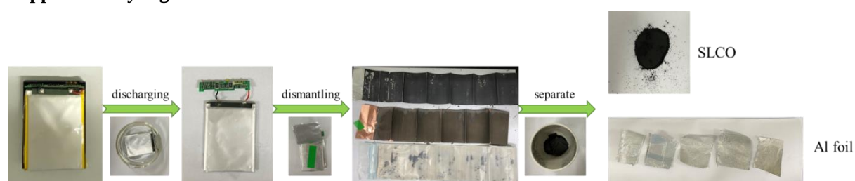
Supplementary Figure 1. Pretreatment of LIBs. Pretreatment steps of spent LIBs.
