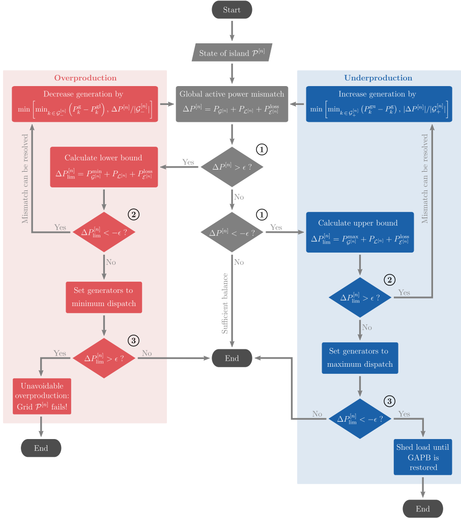
Supplementary Figure 6: The flowchart describing the applied algorithm to restore Global active power balance (GAPB) based on primary frequency control (PFC).
