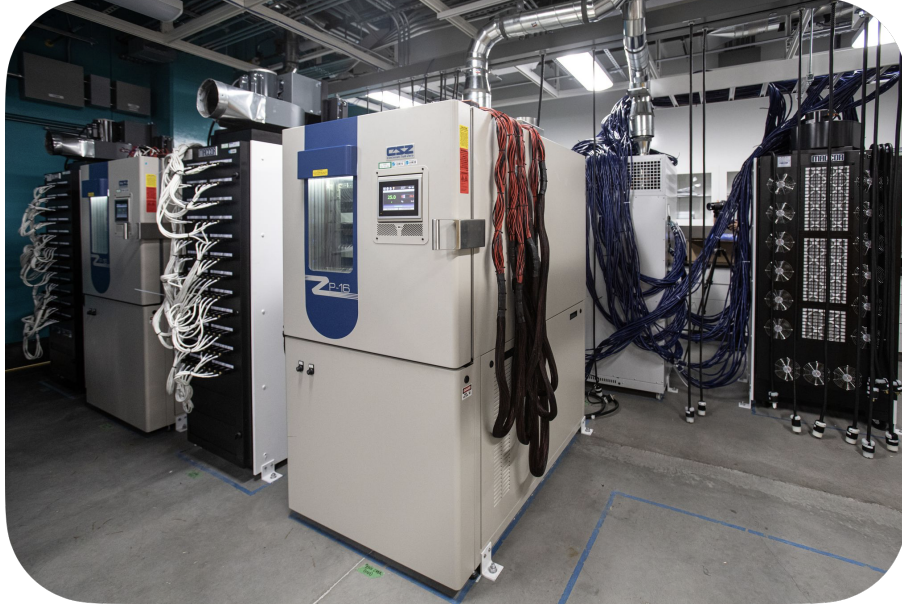
Supplementary Figure 13: Photos of battery cyclers used for battery cycling experiments. The photo shows the CSZ temperature chamber (front-most object, off-white instrument with blue marking in the middle) and Maccor battery cycler (directly to the left, black instrument with white cables coming out) used for the experiments.
