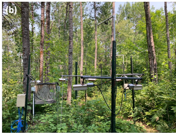
Supplementary Fig. 7. The pictures of plots from the B4WarmED project. (a): the plot of + 3.3 °C under the open canopy; (b): the plot of + 3.3 °C under the closed canopy; (c): the rainout shelter that was installed to remove rainfall under the open canopy; (d): the PVC collar that was used to measure soil respiration. The height of the infrared lamp heater was approximately 1.6 m. All photos were taken by Guopeng Liang in June of 2023.
