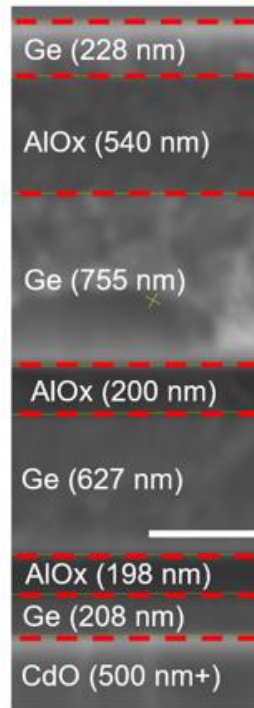
Fig. S3. XSEM image of the 7-layer sample in Fig. 2d. The scale bar is 500 nm.
