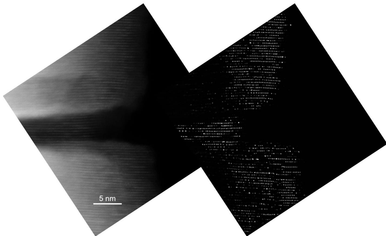
Figure S8. Demonstration of atom segmentation and localization by AtomSegNet . The left panel shows an atomic resolution high-angle annular dark-field scanning transmission electron microscopy (HAADF-STEM) image of a delithiated NMC-811 particle. The right panel shows the AtomSegNet -processed super-resolution image corresponding the image in the left panel.
