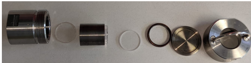
Supplementary Figure 151. Photograph of the disassembled autoclave including quartz glass lining.
