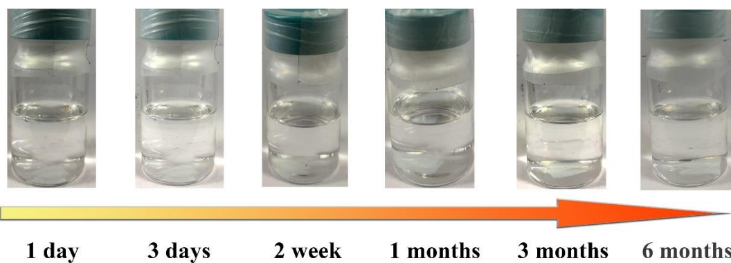
Supplementary Figure 12 | Immersing the MOF-gel separator in electrolyte over 6 months. It retained stable morphologies in electrolyte.
