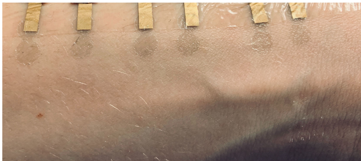
Fig. S19. Original optical image of 6 graphene electronic tattoos placed over subject's radial artery, the same image as used in main manuscript, Fig. 1c.
