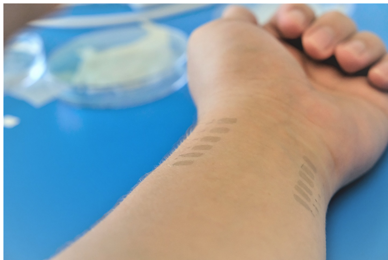
Fig. S20. Optical image of 12 graphene electronic tattoos plainly placed over subject's ulnar and radial arteries.
