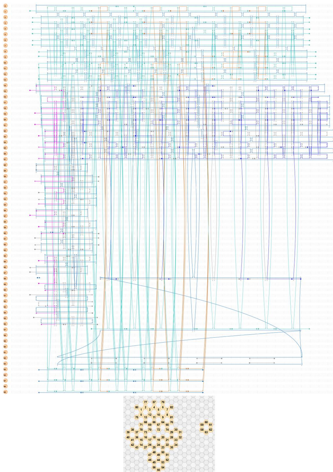
Figure S22. caDNAno design of the DNA origami in the DOS variant with blocked central channels in the needle. The cross-section of the structure is shown at the bottom of the strand diagram. Both were generated using caDNAno. The filled hexagonal lattice follows previous designs 2 , and the use of short miniscaffold strands to overcome scaffold length limitations is adapted from prior work. 3
