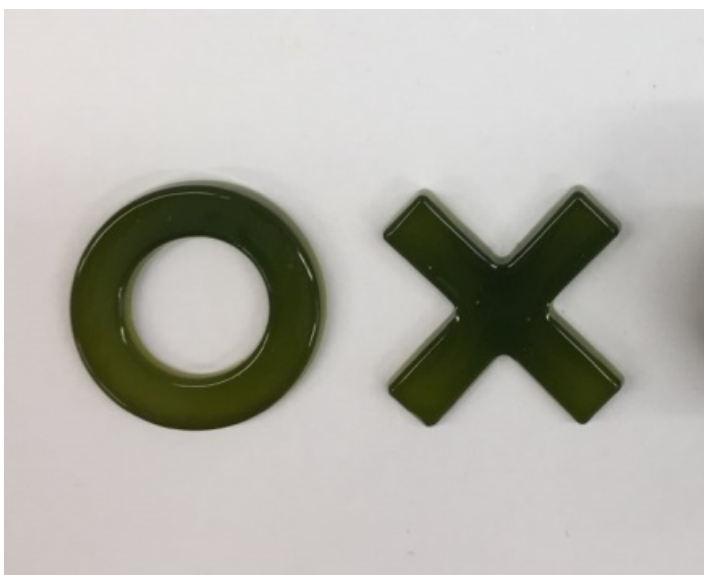
Figure S4. Silicone mold filled with gel reaction mixture, irradiated with NIR lamp through silicone barrier, yielded defined X and O PMMA gels.
