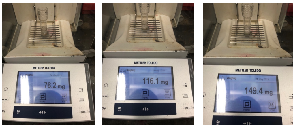
Left: \text{AgPF}_6 (76 mg). Center: n\text{Bu}_4\text{NPF}_6 (116 mg). Right: 3\text{ \AA} MS (150 mg).
