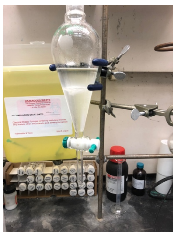
Left: dilute with \text{Et}_2\text{O} (30 mL) and washed with sat. \text{NH}_4\text{Cl} (aq). Center: washed with brine. Right: dried over \text{Na}_2\text{SO}_4 and filtered.
