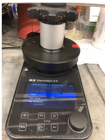
Left: no need to use a reference electrode. Center: choose “Time”. Right: set reaction time to 3h.
