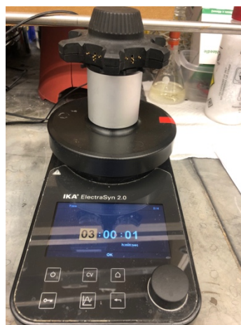
Left: no need to use a reference electrode. Center: choose “Time”. Right: set reaction time to 3h.
