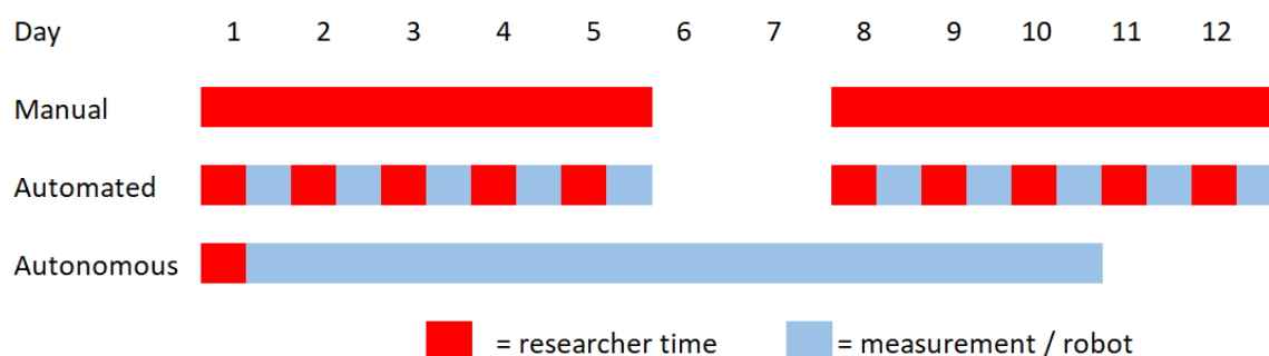
Figure S31. Comparison of the time needed to carry out 1000 photocatalysis experiments using different methodologies, assuming a 5-day working week. For the manual method, it is possible to carry out two experiments per day, requiring 500 days of researcher time (700 days total, assuming a 5-day work week). Using a semi-automated (but not autonomous) robotic method that we developed previously (ref. 33 in main text), we can carry out 100 experiments per day. This semi-automated method requires half a day of researcher time to set it up, so 1000 experiments requires 5 days of researcher time (12 days of experiment in total; see figure). The new autonomous approach developed here also requires a half-day set up, but then the experiment runs independently, 24/7, without any user input. As such, the autonomous workflow is 500–1000 times faster than manual approaches, and at least 10 times faster than semi-automated robotic methods based on dedicated researcher time. The true efficiency gains are larger than this because in the semi-automated method, the researcher would need to retrieve the results of the last batch of experiments and manually apply a process or algorithm to decide on the next batch. In the autonomous workflow, this is done (effectively) instantaneously. Furthermore, 100 experiments per batch is non-optimal from the perspective of batched Bayesian optimization, but a reduction in the batch size for the semi-automated experiment would reduce the throughput significantly. This is because the time saving in that method arises from batched photolysis and analysis of a large number of samples at one time (100), thus reducing the number of manual loading and unloading operations. In principle, we could operate the workflow illustrated in Supplementary Movie S3 at the same speed by using a human researcher to convey the samples from station to station, but we note that this would be an unappealing prospect (8 days of continuous work 24/7) and subject to user error ( e.g. , the robot makes 4816 independent sample vial transfers during the 8-day experiment, all of which must occur in the correct sequence).
