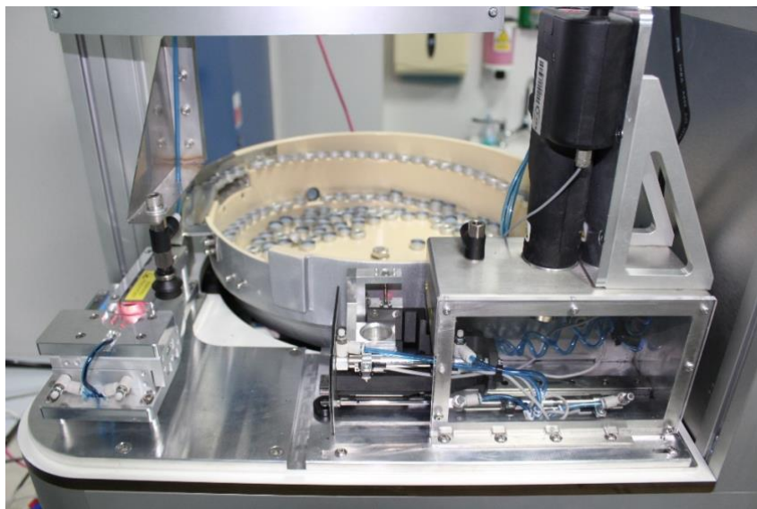
Figure S21. Photograph of the Liverpool Inertization Capper-Crimper (LICC). The bowl feeder that contains a stock of vial caps can be seen in the rear. The inertization chamber is in the lower right of the photograph and has a plastic window at the front to allow observation of the capping process in case of failure (see also section 9 on 24/7 monitoring). The crimper itself is the black, vertically-mounted instrument in the top right of the photograph.
