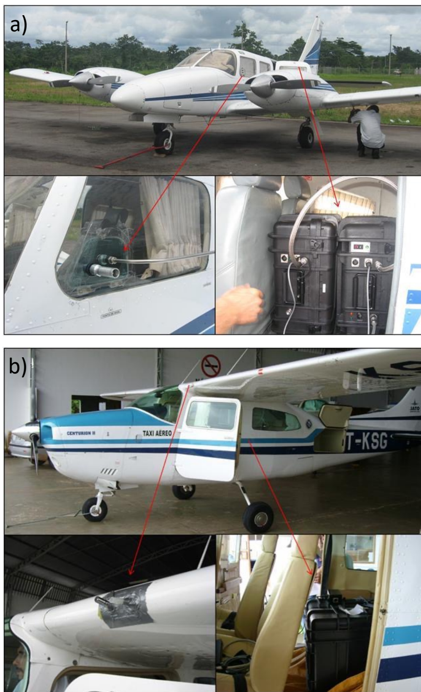
Supplementary Information Fig. 5 | Sampling details installation. a) Twin-engine aircraft used at RBA, showing in detail the inlet in the inspection window (curved stainless steel tube) and temperature and relative humidity (T & H) sensor and the PCP (Portable Compressor Package) and PFP (Portable Flask Package) installed in the aircraft. b) Single-engine aircraft used at ALF, where the inlet and T & H sensor is installed in the wing and the PCP and PFP are behind the pilot's seat)
