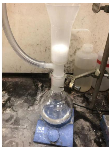
(Left) Combined organic layers were dried over \text{Na}_2\text{SO}_4 . (Center) Filtration to remove \text{Na}_2\text{SO}_4 . (Right) Solvent removal under reduced pressure.
