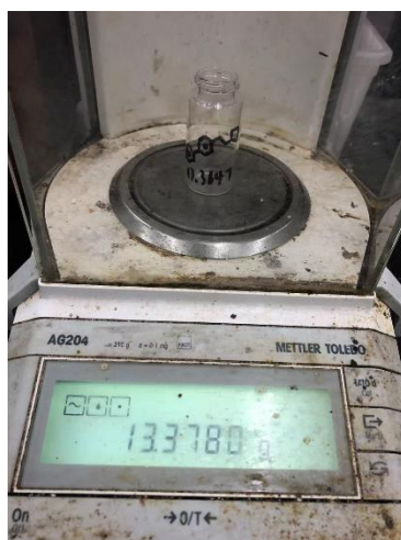
(Left) Crude TLC (10:1 Hexanes: EtOAc). (Center) Purification by pTLC (10:1 Hexanes: EtOAc). (Right) Tared weight of vial containing desired product (13.3 mg, 51% yield).
