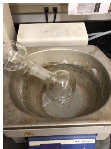
(Left) Combined organic layers were dried over \text{Na}_2\text{SO}_4 . (Center) Filtration to remove \text{Na}_2\text{SO}_4 . (Right) Solvent removal under reduced pressure.
