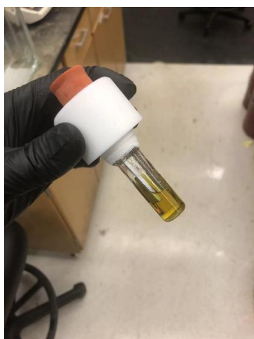
(Left) Reaction mixture after electrolysis. (Center) Electrodes were rinsed with \text{Et}_2\text{O} and entire reaction mixture was transferred to a separatory funnel with \text{Et}_2\text{O} . The organic phase was washed with 0.1N HCl (aq). (Right) Combined organic layers were washed with brine (NaCl).
