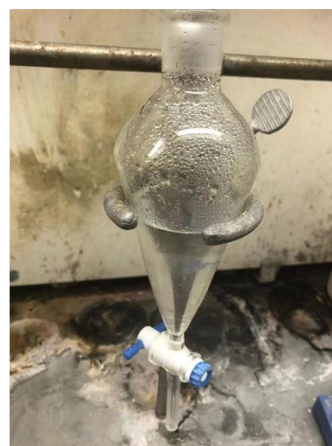
(Left) Reaction mixture after electrolysis. (Center) Electrodes were rinsed with \text{Et}_2\text{O} and entire reaction mixture was transferred to a separatory funnel with \text{Et}_2\text{O} . The organic phase was washed with 0.1N HCl (aq). (Right) Combined organic layers were washed with brine (NaCl).
