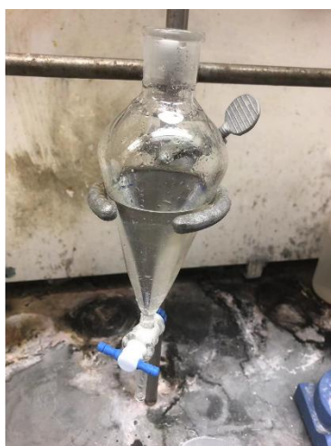
(Left) Reaction mixture after electrolysis. (Center) Electrodes were rinsed with \text{Et}_2\text{O} and entire reaction mixture was transferred to a separatory funnel with \text{Et}_2\text{O} . The organic phase was washed with 0.1N HCl (aq). (Right) Combined organic layers were washed with brine (NaCl).
