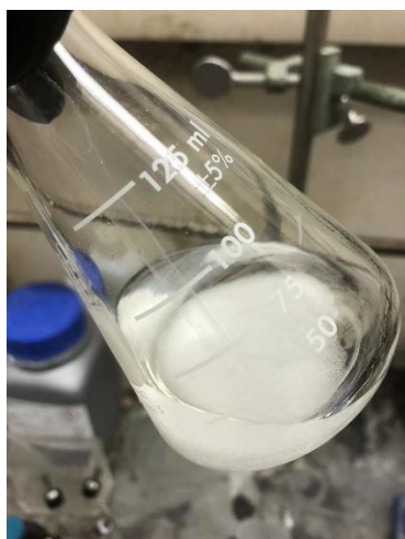
(Left) Combined organic layers were dried over \text{Na}_2\text{SO}_4 . (Center) Filtration to remove \text{Na}_2\text{SO}_4 . (Right) Solvent removal under reduced pressure.
