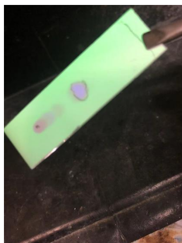
(Left) Crude TLC (10:1 Hexanes: EtOAc). (Center) Purification by pTLC (10:1 Hexanes: EtOAc). (Right) Tared weight of vial containing desired product (13.3 mg, 51% yield).
