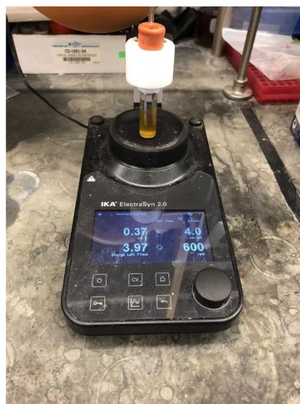
(Left) Complete setup of reaction prior to electrolysis. (Right) Reaction setup during electrolysis ( note: 600 rpm stirring ).
