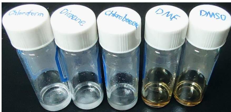
Fig. S3. Pictures of H-BFDO in different solvents ( 15 \text{ mg ml}^{-1} ) after being heated at 100^\circ\text{C} for 30 min (H-BFDO exhibited better solubility in DMF/DMSO than that in chlorobenzene/dioxane/chloroform.).
