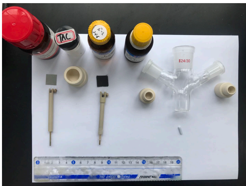
Fig. S1 Step 1: Materials used for undivided cell set-up.
