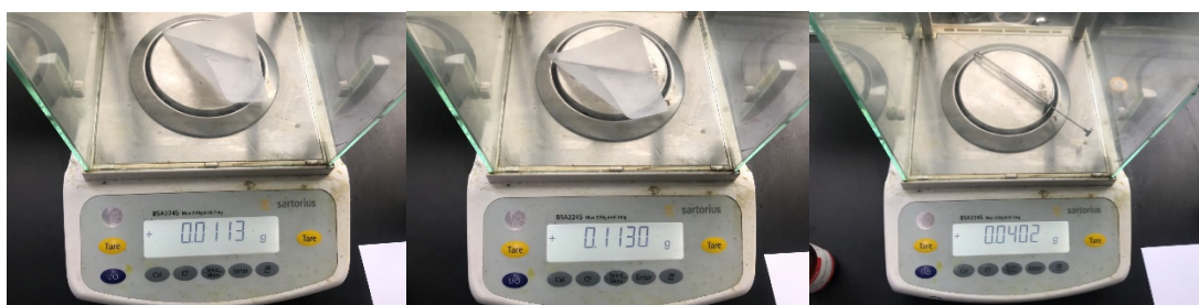
Fig. S3 Step 3: \text{TAC}^+\text{ClO}_4^- (11.3 mg, 0.024 mmol), \text{Et}_4\text{NBF}_4 (113.0 mg, 0.52 mmol, 0.1 M), n -butylbenzene S8 (40.2 mg, 0.3 mmol), added to the cell.
