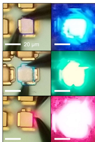
Supplementary Figure 11 | Schematic diagram and optical and EL microscopy images of fully isolated vertical RGB \mu\text{LED} chips.
