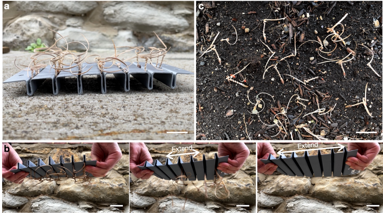
Figure S7. Conceptualized storage and delivery mechanism. a , The assembly of seeds on an extendable accordion structure to avoid entanglement. b , The dropping of the seed through the extension of the seed storage device. c , Seeds delivered and dropped on the ground. Scale bar: 10 mm.
