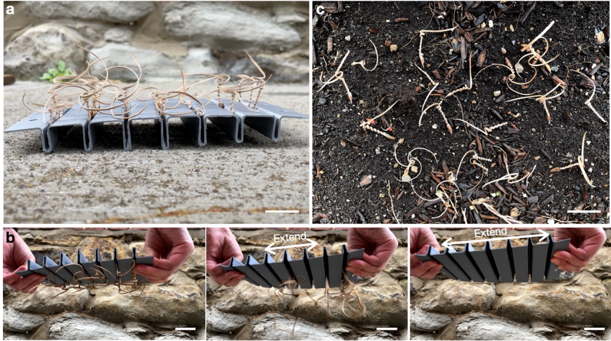
Figure S14. Conceptualized storage and delivery mechanism. a , The assembly of seeds on an extendable accordion structure to avoid entanglement. b , The dropping of the seed through the extension of the seed storage device. c , Seeds delivered and dropped on the ground. Scale bar: 10 mm.
