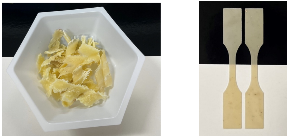
Figure S62. Digital images of LDPE-PLLA (50/50 wt%) + UDC3 (5 wt%) blend extrudate flakes (left) and dogbone tensile specimens generated from reprocessing post-tensile test specimens (right). The original blend of LDPE-PLLA (50/50 wt%) + UDC3 (5 wt%) was first compounded via melt-extrusion, and the blend extrudate was reprocessed via compression molding into dogbone specimens for initial tensile tests. After these tensile tests, the broken pieces were mixed with 50 wt% virgin LDPE and melt-extruded, and the resulting blend extrudate (now 75/25 wt% LDPE-PLLA + 2.5 wt% UDC3) was once again compression-molded to the reprocessed/recycled dogbone specimens (right image) for additional tensile tests. The results were reported in Figure S65.
