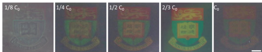
Fig. R3 | performance of photonic nanoswarm with different concentrations of the particle mixture. Scale bar: 2 mm.
