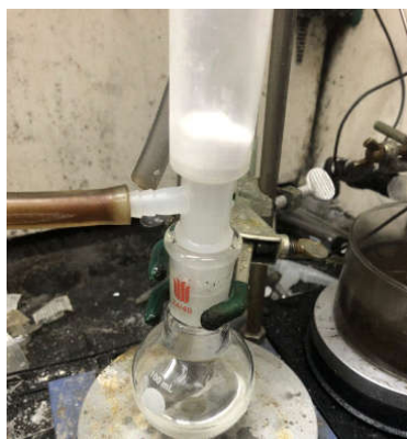
(Left) Combined organic layers were dried over \text{Na}_2\text{SO}_4 . (Center) Filtration to remove \text{Na}_2\text{SO}_4 . (Right) Solvent removal under reduced pressure.
