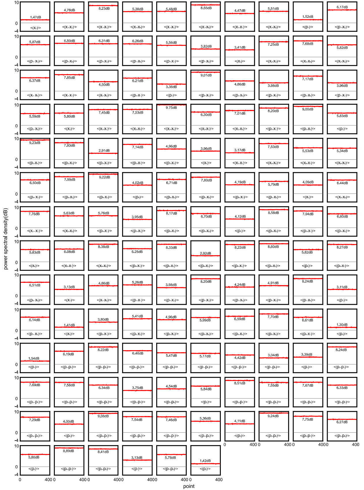
Figure S6 A full set of experimentally measured paired quadrature correlations. Bichromatic homodyne detections were implemented to characterize quadrature correlations between paired frequency combs. All traces have been normalized to the vacuum noise levels that were measured by performing monochromatic homodyne detections. The quadrature components x and p were measured by adjusting the wave-shaper to rotate the LO light with a 0 and \pi/2 phase, respectively. Switching of LOs was enabled by operating the wave-shaper, and LOs were adjusted to the same power by controlling the wave-shaper. All data were collected at the 5 MHz sideband frequency.
