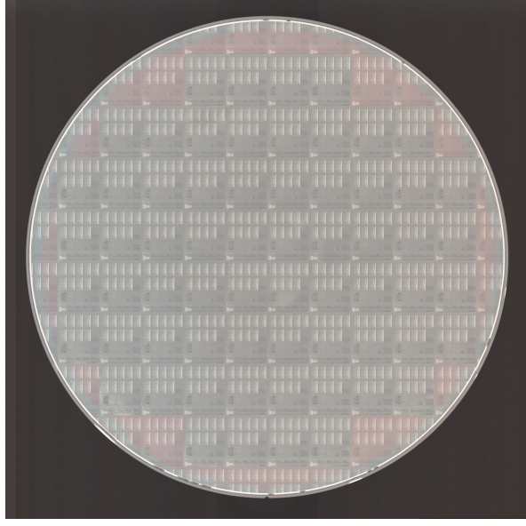
FIG. S15: Example wafer. Photograph of a representative 300 mm wafer fabricated on the customized process used to yield chips for this experiment.
