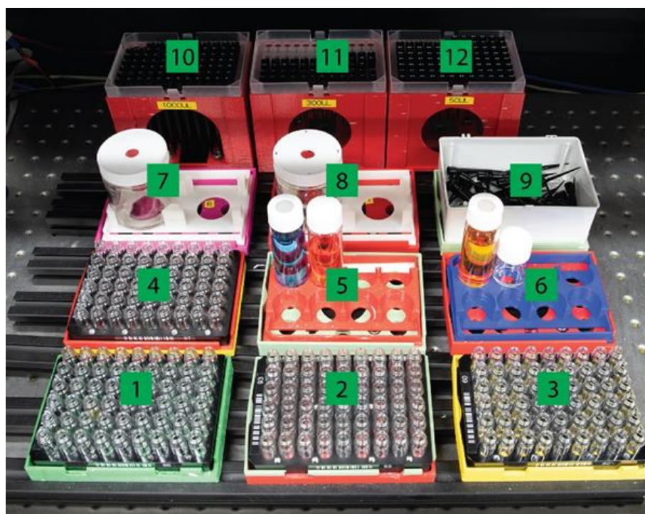
Figure S13. Arrangement of items on the breadboard. 1, 2, 3, 4: slots for well plates. 4, 5: slots for stock solution in 20 mL bottles. 7, 8: slots for stock solution in 100 mL jars. 9, tip trash can. 10, 11, 12: tip racks for tips of 1000 \mu L, 300 \mu L and 50 \mu L, respectively. All holders or racks are 3D printed, and the well plates are CNC machined. The CAD files for machined plates and 3D printed parts can be found the Zenodo data archive associated with this paper – specifically, in the directories “mechanical_designs\well_plates” and “mechanical_designs\holder_for_plates”.
