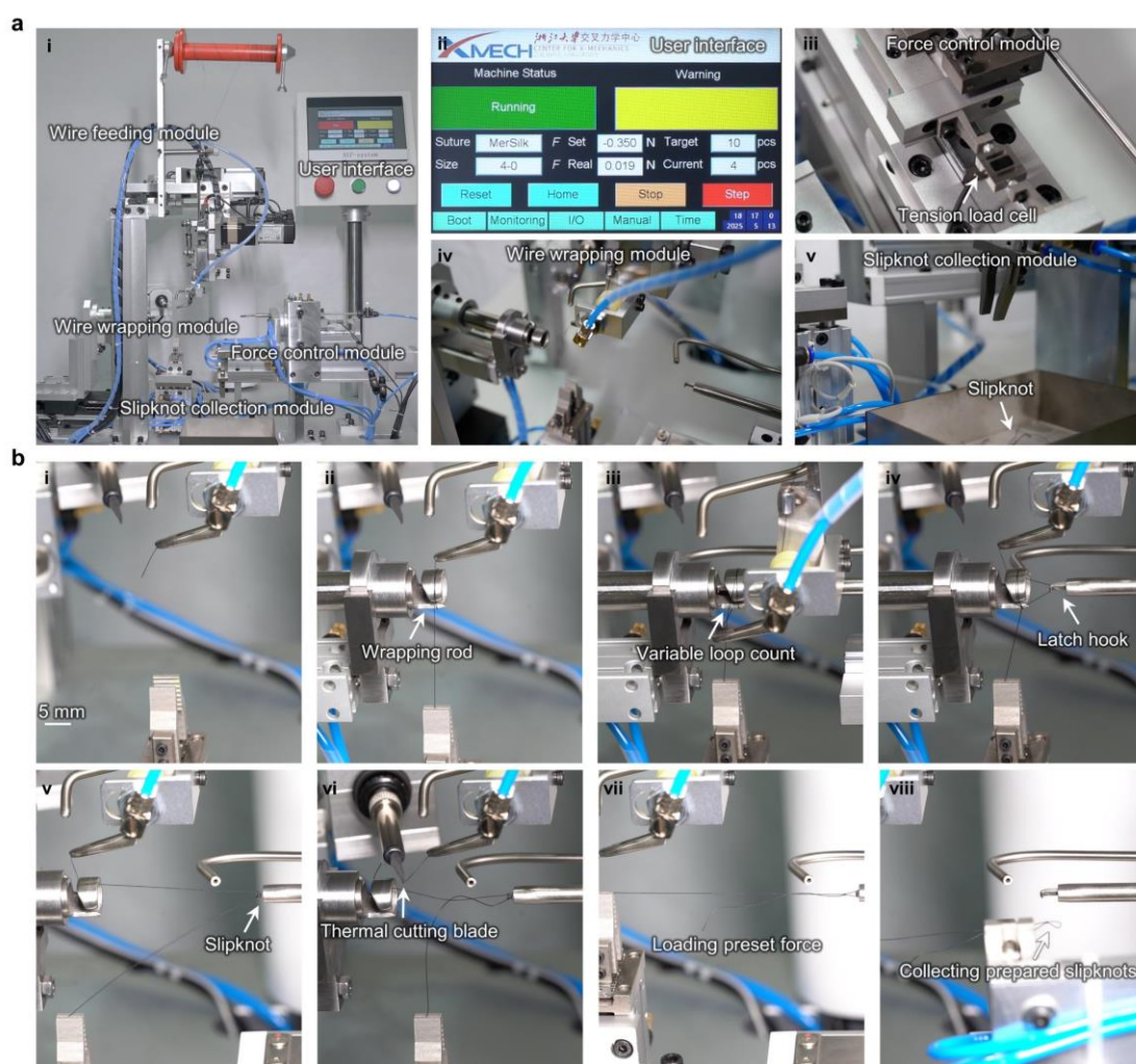
Fig. R11 (added in revised Supplementary Materials as Supplementary Fig. 21): Automatic slipknot fabrication machine. a, (i) Overall view of the system, which integrates modules of wire feeding, force control, wire wrapping, slipknot collection,
