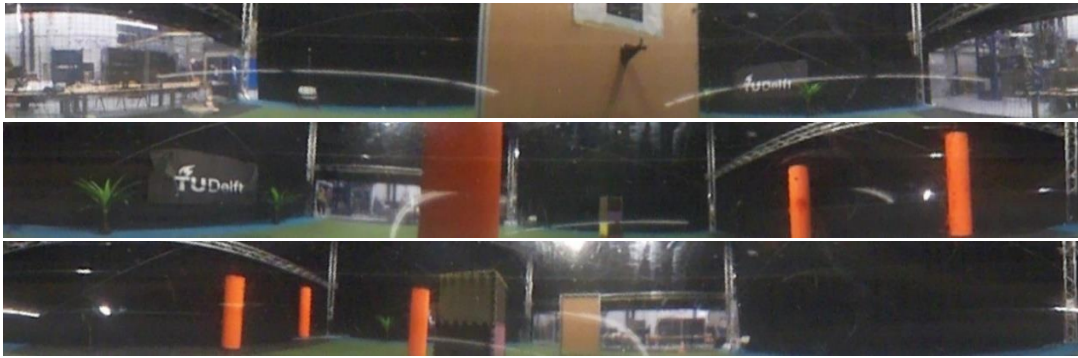
Figure SI-19: Three onboard images captured directly in front of the obstacles. Although the center of the panoramic view is blocked, the wide angle of view provides sufficient surroundings to perform homing predictions. This allows for the correct vector predictions shown in the previous figure.
