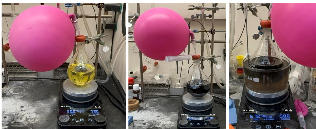
(Left) reaction mixture after DMSO addition. (Center) reaction mixture after TMG addition. (Right) reaction mixture was stirred at 70 °C overnight.
