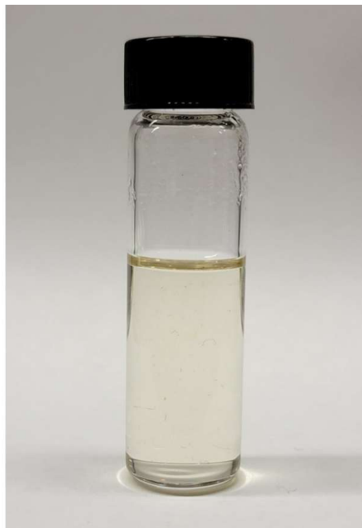
Figure S39. Solubility test of the solid product after the PVC upcycling reaction using \text{FeCl}_3 . (left) Representative powder of the solid product. (right) A solution of the solid product (35 mg) in 1,2,4-trichlorobenzene (7 ml).
