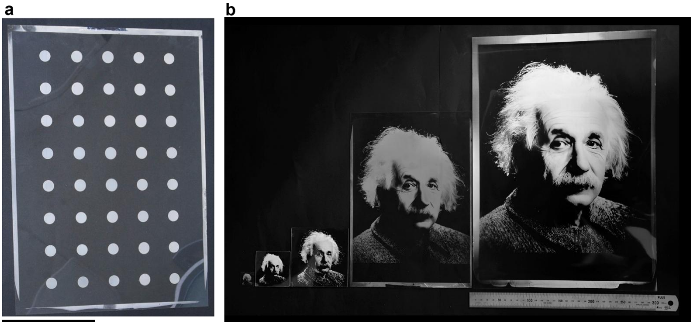
Supplementary Fig. 29 | Scale-up demonstration of the DFP process and test of print uniformity. a , Photograph of A4 printing of circular dots. Scale bar, 10 cm. The PS/THX film was illuminated using a large LED array (Micro Square Co., Ltd, \lambda_i : 385 nm) with an energy dose of 150\text{ J cm}^{-2} . The illuminated film was developed at 32^\circ\text{C} acetic acid for 1 min. b , Scale-up printing of the photo Albert Eistein (Original photo by Oren Jack Turner, Princeton, N.J.), where the samples \leq 10\text{ cm} \times 10\text{ cm} were made by spin casting and illuminated using a UV projector ( \lambda_i : 405 nm) or using custom LED chamber (Thorlabs, \lambda_i : 405 or 385 nm), while the samples > 10\text{ cm} \times 10\text{ cm} were made by bar coating and illuminated using a large LED array (Micro Square Co., Ltd, \lambda_i : 385 nm). The substrate for A4 and A3 specimen is 188\text{-}\mu\text{m} -thick PET sheet (Lumirror T60, Toray Industries, Japan) and OHP film ( 0.1\text{-mm} -thick polyester film, Sakae Technical Paper Co., Ltd., Japan), respectively. Ruler for scale (cm).
