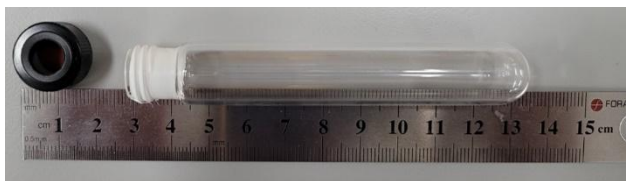
Supplementary Figure 1. Reaction test tube (12 mL, 15 mm × 100 mm). (Samwoo Kurex, Borosilicate, Type 1 glass).
