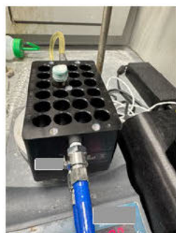
placement of vial in Lumidox
