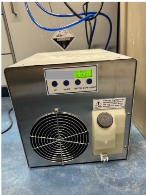
Figure S1.3. External cooling setup for temperature-controlled irradiation.
