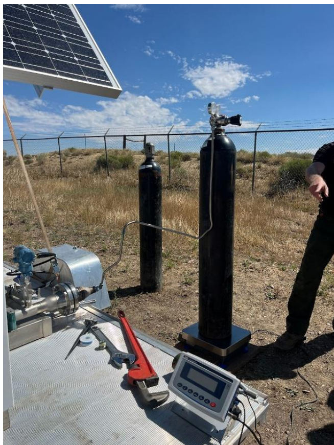
Figure S84. Field site Coriolis meter calibration with gas cylinder on scale.
