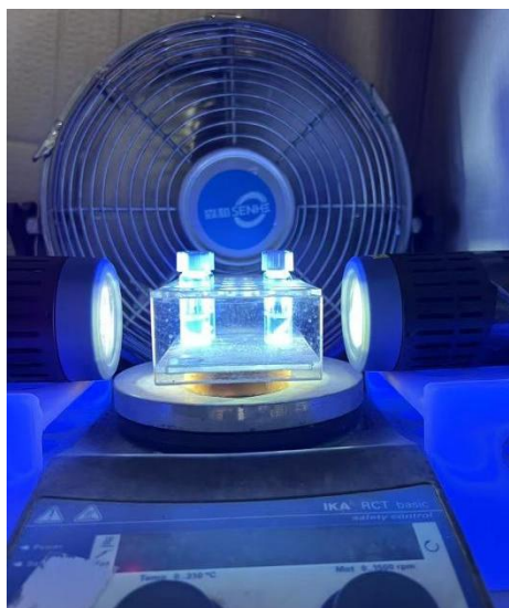
Supplementary Figure 1. Reaction set-up (Left: 40 W LEDs, Right: 40 W LEDs; \lambda_{\text{max}} = 370 \text{ nm} ). (The fan is used to keep the reaction temperature being around room temperature \sim 25^\circ\text{C} )
