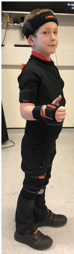
Figure 1 (left): the high resolution “suit” system, example of how the sensors can be placed with elastic straps. (right) Avatar reconstruction of movement.
