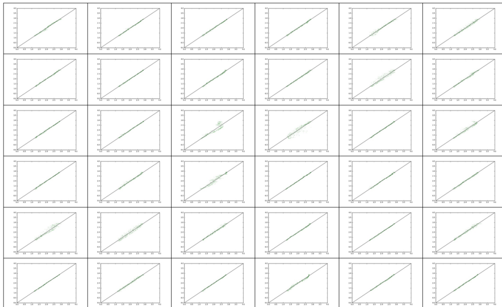
Figure S3 (b). Predicted vs measured displacement after the data transformation based on the regression result, showing the perfect coincidence between the predicted and measured displacement for every sector.
