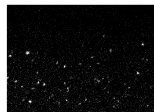
h. SEM-EDS map for Ca, Ka showing a fairly homogenous distribution of calcium with a few larger clusters.
