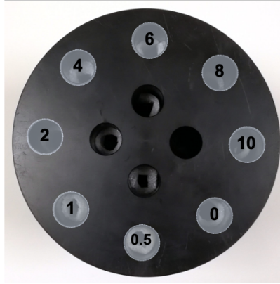
Supporting Figure 1: A phantom setup for the SPCCT scanner. Tubes with the concentrations of AuNP noted (in mg/mL) suspended in 1% agarose gel were placed in the outer eight holes.
