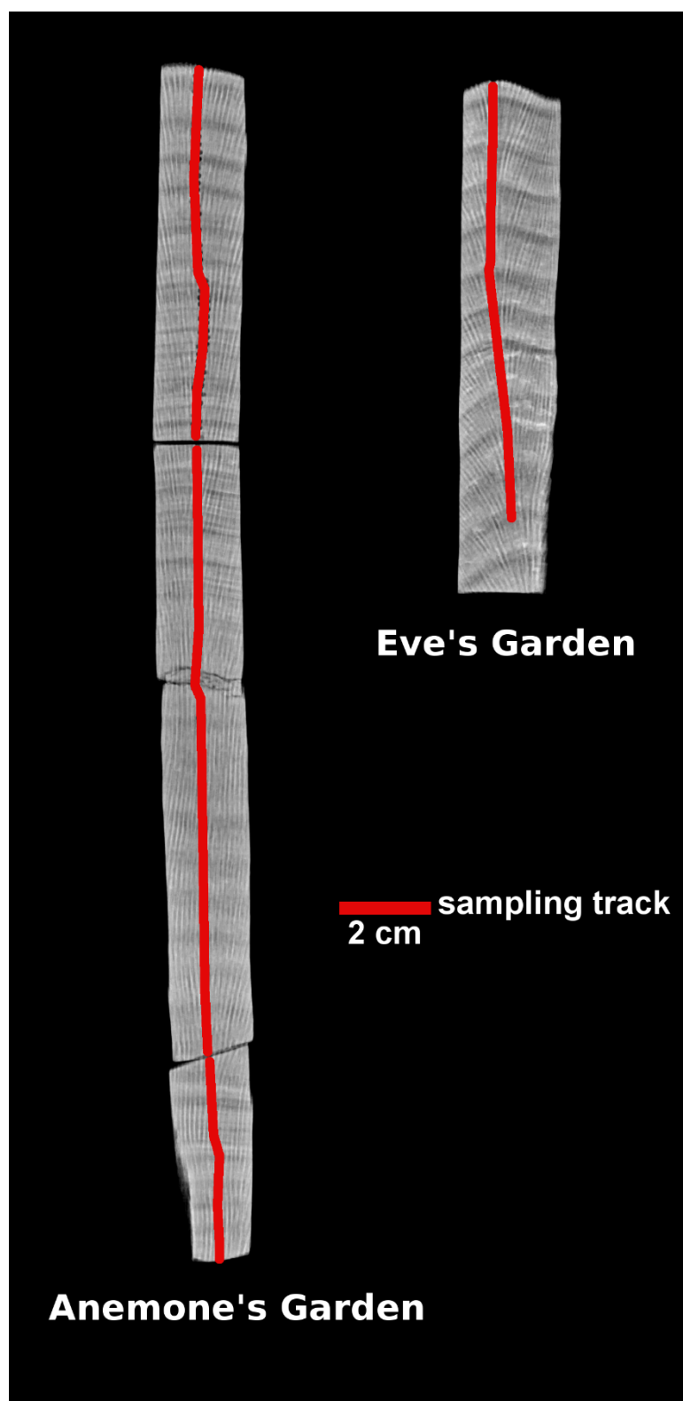
Figure S4 - X-ray images of coral cores with sampling tracks marked in red.
