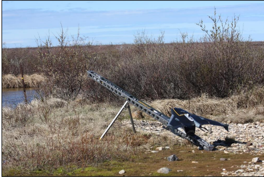
Figure S1.3. The UX5 mounted on its elastic catapult launcher.
